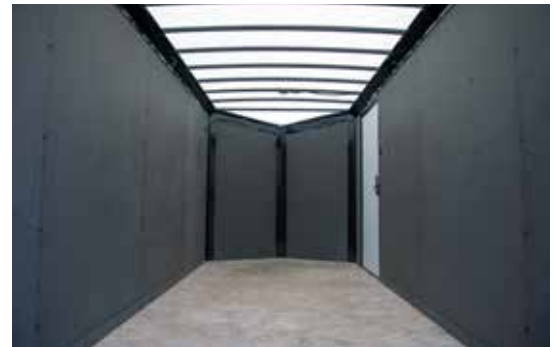
Great Combo: New Engineered Fibre Panel (EFP) & translucent LightLid available as optional equipment
